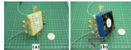
Development of the miniature Air-breathing PEMFC Stack
