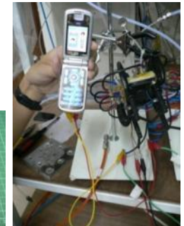
Development of the miniature Air-breathing PEMFC Stack
