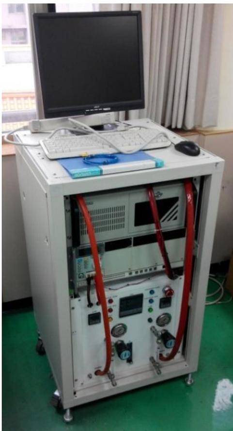
300W Fuel Cell Test Station
